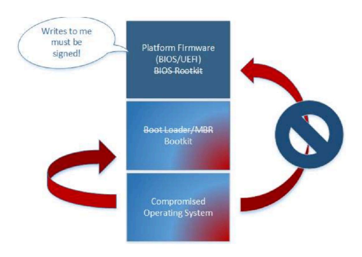
Modern platform implement the requirement that updates to the firmware must be signed. This makes compromising the BIOS with a root kit harder
