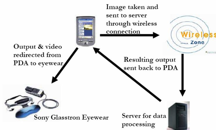
**PDA based mobile architecture for face biometrics that we have implemented and demonstrated.**
