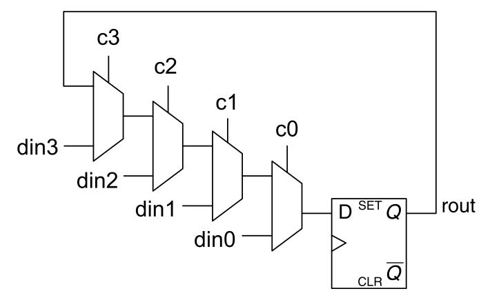
Critical path delay: 4 2x1 MUX.
