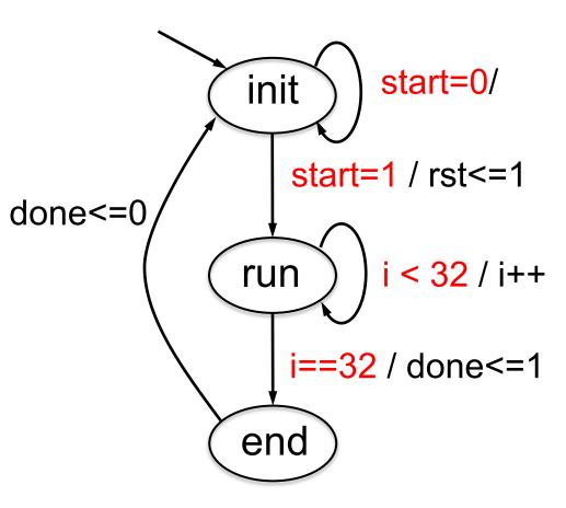
Output logic: in\_addr <= i; out\_data <= ... Input: M[i] Outputs: max, min, average
