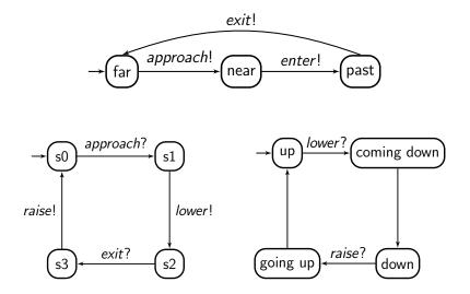
2 or 3 minutes after the train signals the controller *approach*, it reaches the gate. At most 5 minutes after the train signals *approach*, it leaves the gate.
