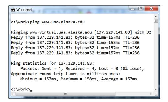
Signal propagates at about the speed of light, which is about 1 nanosecond per foot or 5 microseconds per mile. At 4000 miles one-way the round-trip propagation delay is about 40 milliseconds. Assuming a fairly straight path from Tampa to Anchorage, about 120 millseconds of the shown round-trip delay is not due to propagation. It is most likely due to queueing delays in routers between Tampa and Anchorage.
