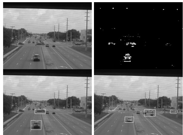
Figure 2: Original image (top left), and regions containing motion with bounded boxes placed over vehicles.
