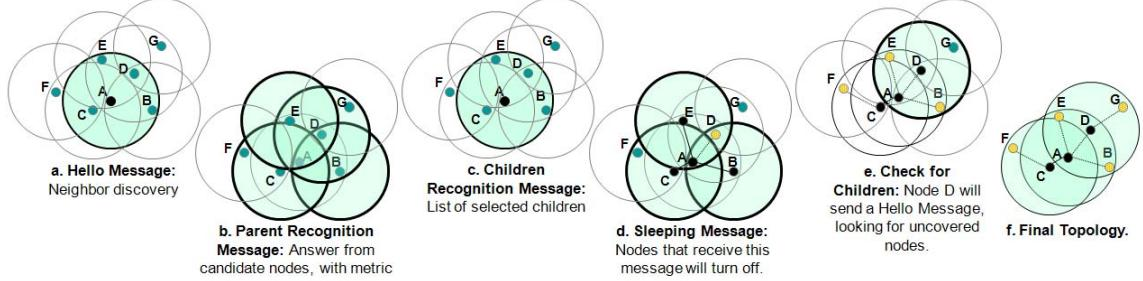
Fig. 1. The A3 Algorithm.
